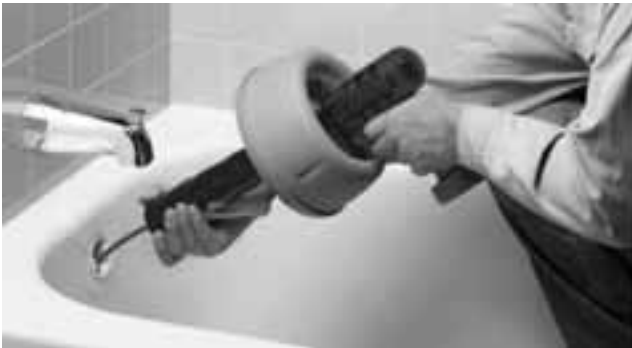
Figure 5 – Keep Distance Between Drain Opening and Nose of Drain Gun to 6" or Less
